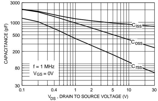
Figure 8. Capacitance Characteristics.
