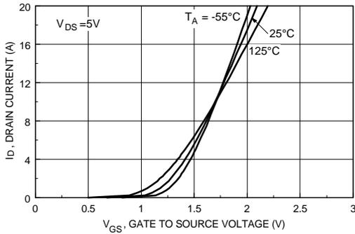
Figure 5. Transfer Characteristics.
