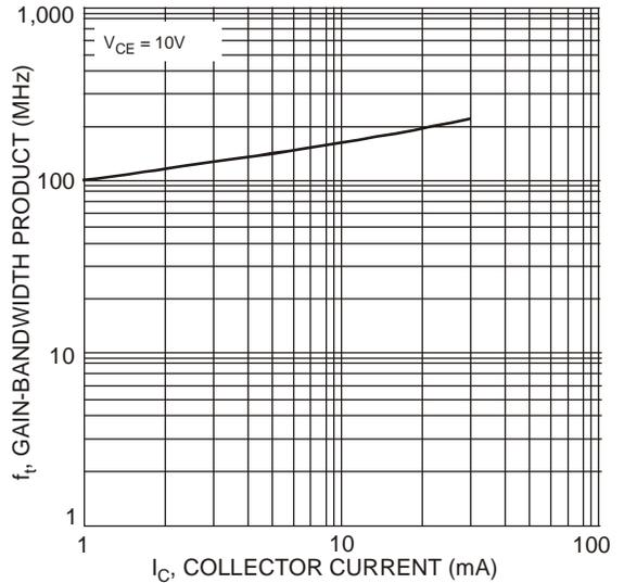
Fig. 4 Typical Gain-Bandwidth Product vs. Collector Current
