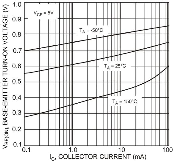
Fig. 3 Typical Base-Emitter Turn-On Voltage vs. Collector Current
