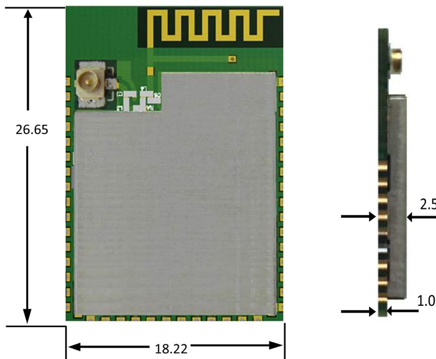
Unit: mm Tolerance: 0.2mm
