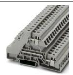
Installation level terminal block, Screw connection, Cross section: 0.2 mm² - 10 mm², AWG: 24 - 8, Width: 8.2 mm, Color: gray, Mounting type: NS 35/7,5, NS 35/15
