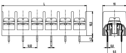
The PCB connector 982-D in 9,52 mm pitch is available in 2- to 26-pole design and can be mounted side-by-side in the nominal pitch. This version is equipped with two solder pins per pole.
