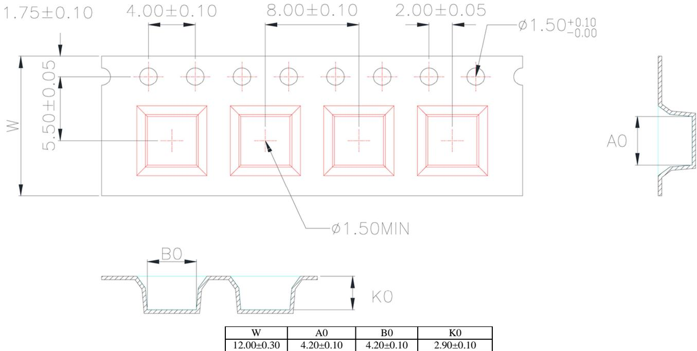
1. 10 sprocket hole pitch cumulative tolerance  $\pm 0.20$ .
