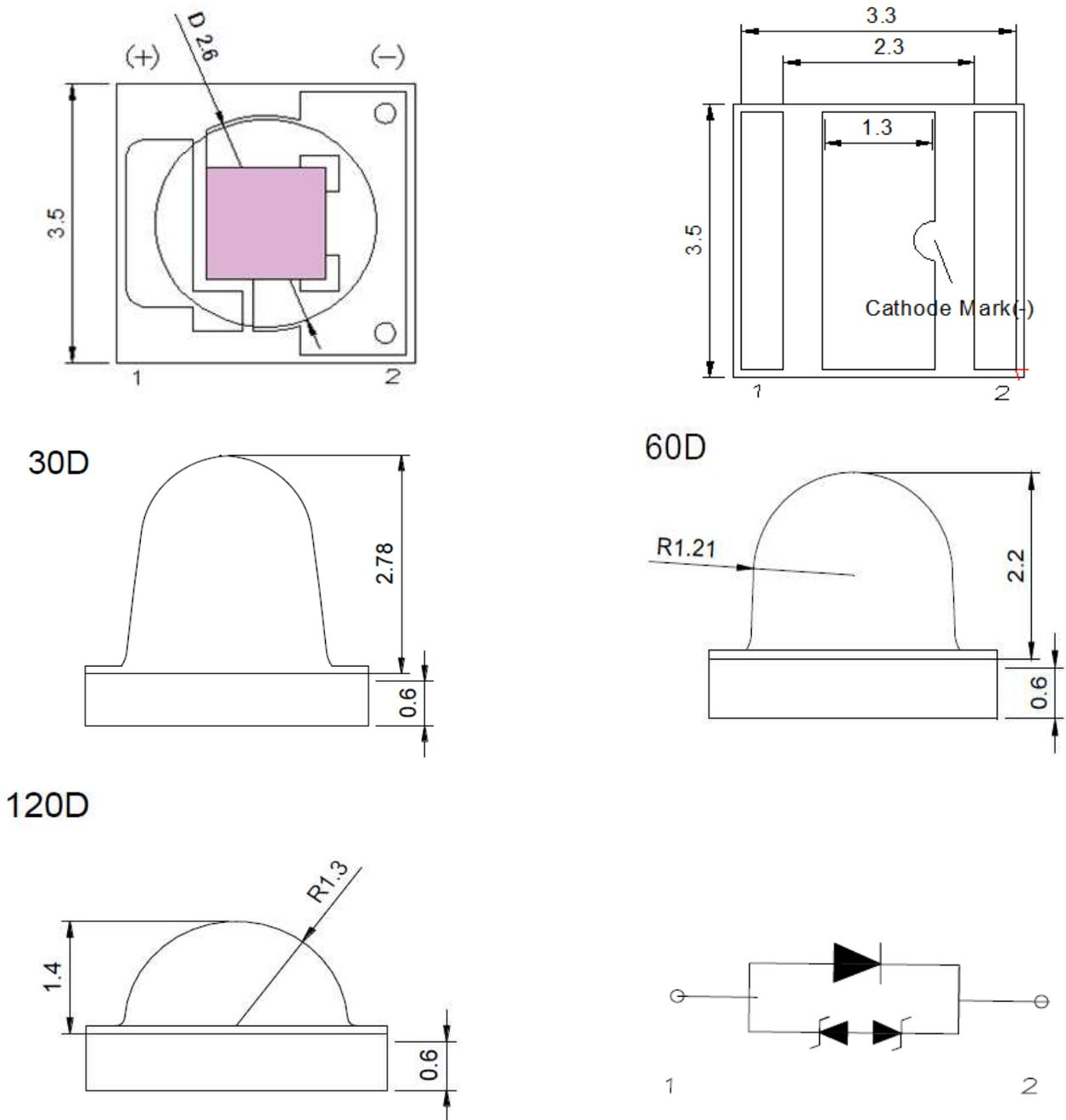
**Figure 2. IN-C33ATN / IN-C33BTN / IN-C33CTN Package Dimension**
