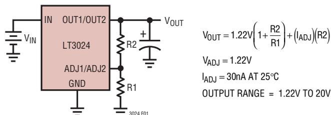
Figure 1. Adjustable Operation
