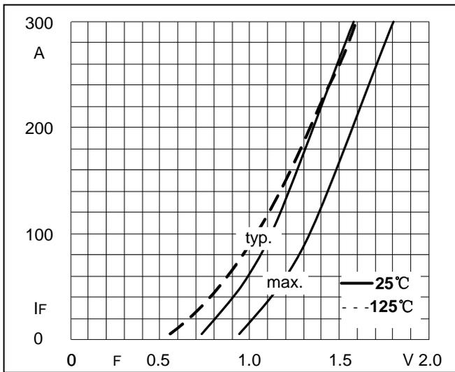
Fig1. Forward Characteristics
