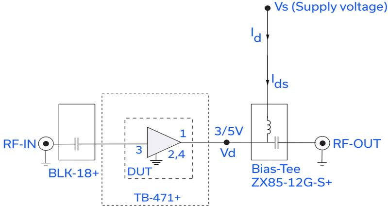
Fig 1. Block Diagram of Test Circuit used for characterization. (DUT soldered on Mini-Circuits Characterization Test Board TB-471+)
