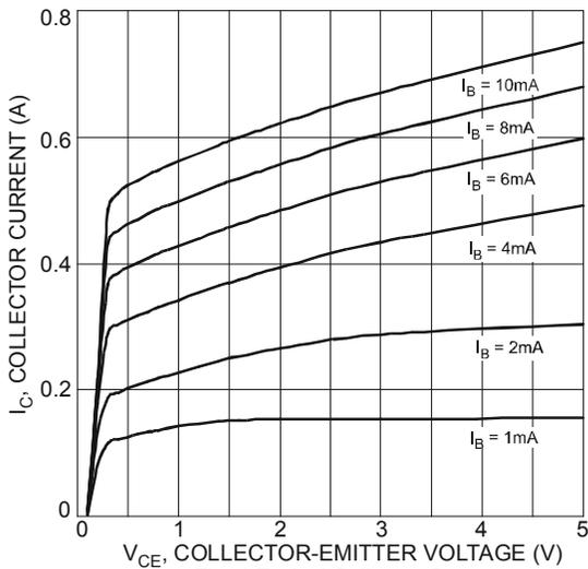
Fig. 1 Typical Collector Current vs. Collector-Emitter Voltage
