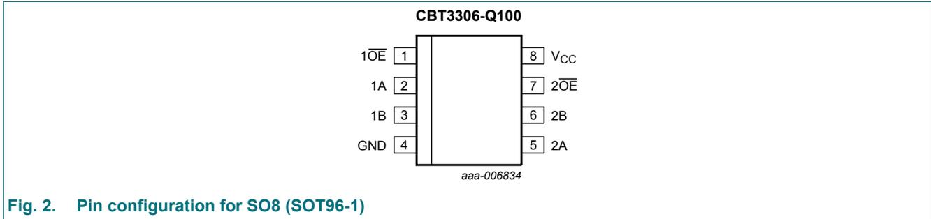
Fig. 2. Pin configuration for SO8 (SOT96-1)
