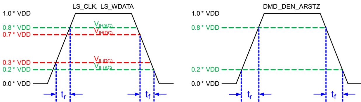
Figure 3. LPSDR Input Rise and Fall Slew Rate
