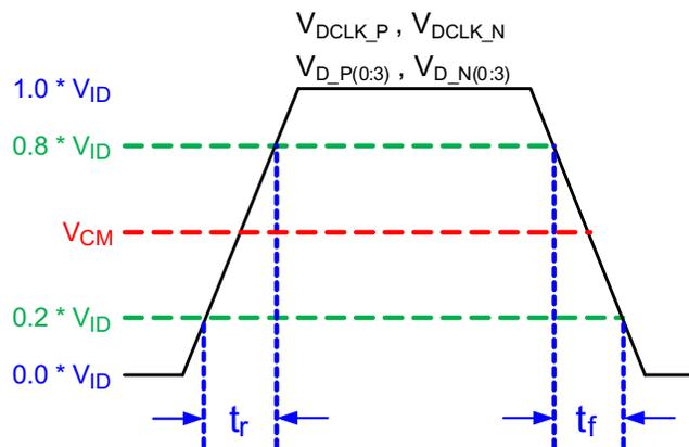
Figure 4. SubLVDS Input Rise and Fall Slew Rate
