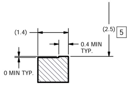
(PANASONIC AXT640124DD1, 40-CONTACT, 0.4 mm PITCH BOARD-TO-BOARD CONNECTOR HEADER) MATES WITH PANASONIC AXT540124DD1 OR EQUIVALENT CONNECTOR SOCKET
