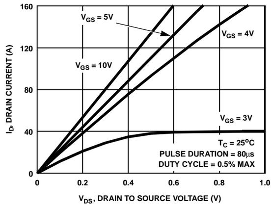
**Figure 8. Saturation Characteristics**
