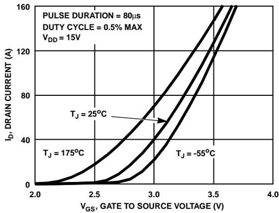
**Figure 7. Transfer Characteristics**
