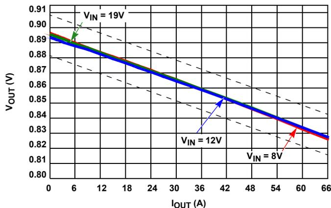
FIGURE 1. LOAD LINE REGULATION
