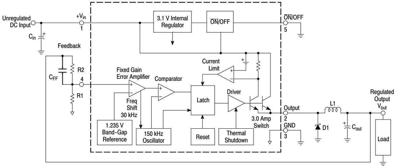
Figure 1. Typical Application and Internal Block Diagram
