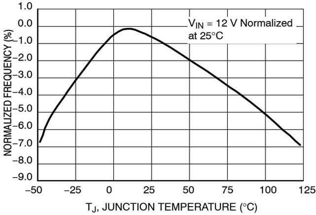
Figure 10. Switching Frequency
