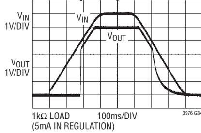
**Burst Mode Switching Waveforms**
