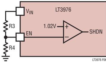
Figure 6. Undervoltage Lockout
