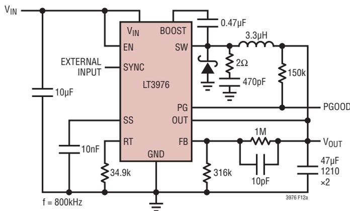
**Figure 12a. Fault Tolerant for  $V_{OUT} < 6V$**
