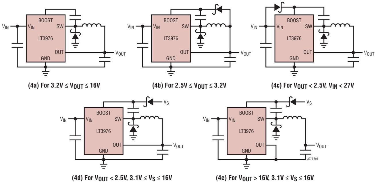
Figure 4. Five Circuits for Generating the Boost Voltage
