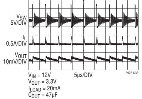
**Full Frequency Switching Waveforms**
