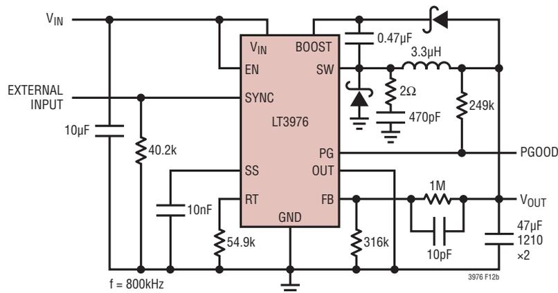
**Figure 12b. Fault Tolerant for  $V_{OUT} < 27V$**
