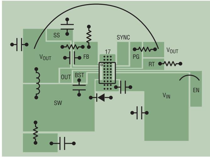
Figure 10. Layout Showing a Good PCB Design
