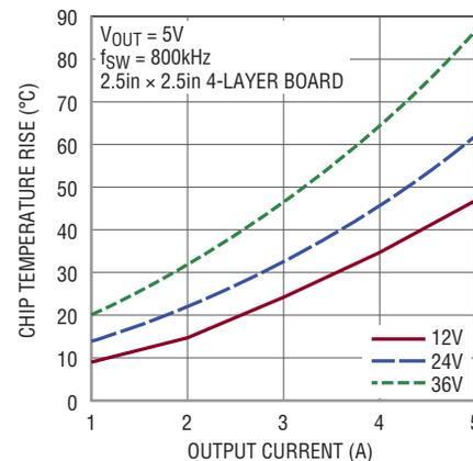
Figure 11b. Temperature Rise of the LT3976 in a 5V<sub>OUT</sub> Application
