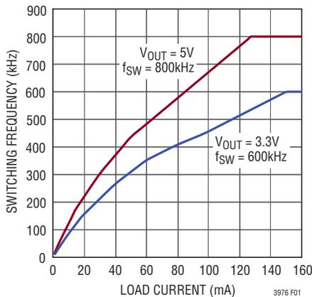
Figure 1. Switching Frequency in Burst Mode Operation
