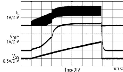
Figure 7. Soft-Start Waveforms for the Front-Page Application with a 10nF Capacitor on SS. EN Is Pulsed High for About 7ms with a 1.65Ω Load Resistor
