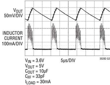
**$V_{OUT}$  and  $I_{IN}$  During Soft-Start**
