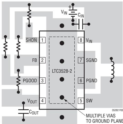
Figure 2. Recommended Component Placement for Single Layer Board
