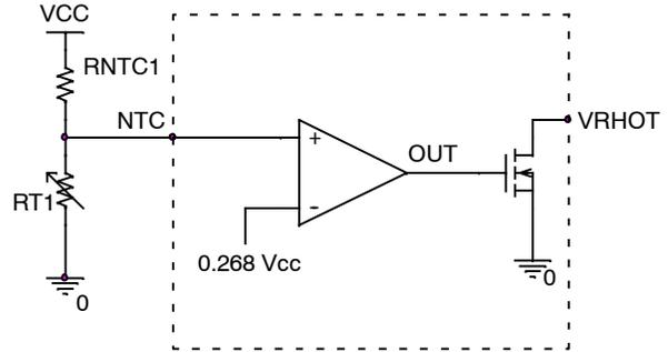
Figure 21. VRHOT Circuit
