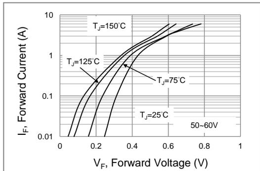
**Fig.6 Typical Forward Characteristics**
