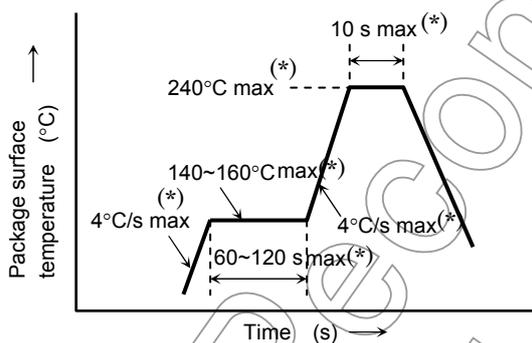
Temperature profile for Pb-free soldering (example)
