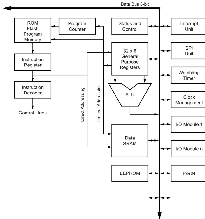
In order to maximize performance and parallelism, the AVR uses a Harvard architecture — with separate memories and buses for program and data. Instructions in the program memory are executed with single-level pipelining. While one instruction is being executed, the next instruction is prefetched from the program memory. This concept enables instructions to be executed in every clock cycle. The program memory is in-system reprogrammable flash memory and ROM.
