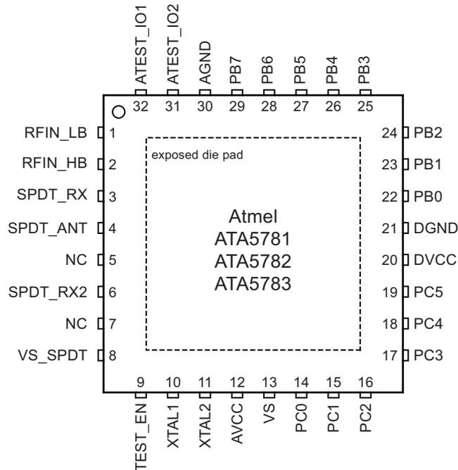
Note: The exposed die pad is connected to the internal die.
