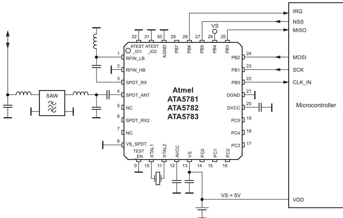
Figure 1-3 shows a typical vehicle side application circuit with an external host microcontroller running from a 5V voltage regulator. The pin PB4 (PWRON) is directly connected to VS and the Atmel® ATA5781/2/3 enters the IDLEMode after power-on. In this configuration the Atmel ATA5781/2/3 can work autonomously and the microcontroller stays powered down to keep current consumption low while remaining sensitive to RF telegrams.
