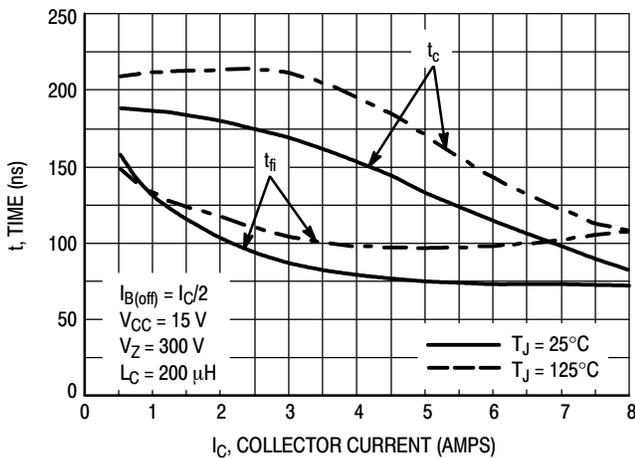
Figure 11. Inductive Switching,  $t_c$  and  $t_{fi}$
