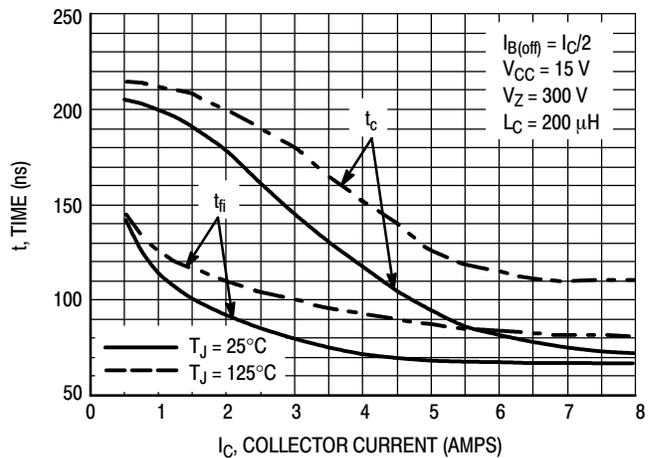
Figure 12. Inductive Switching,  $t_c$  and  $t_{fi}$
