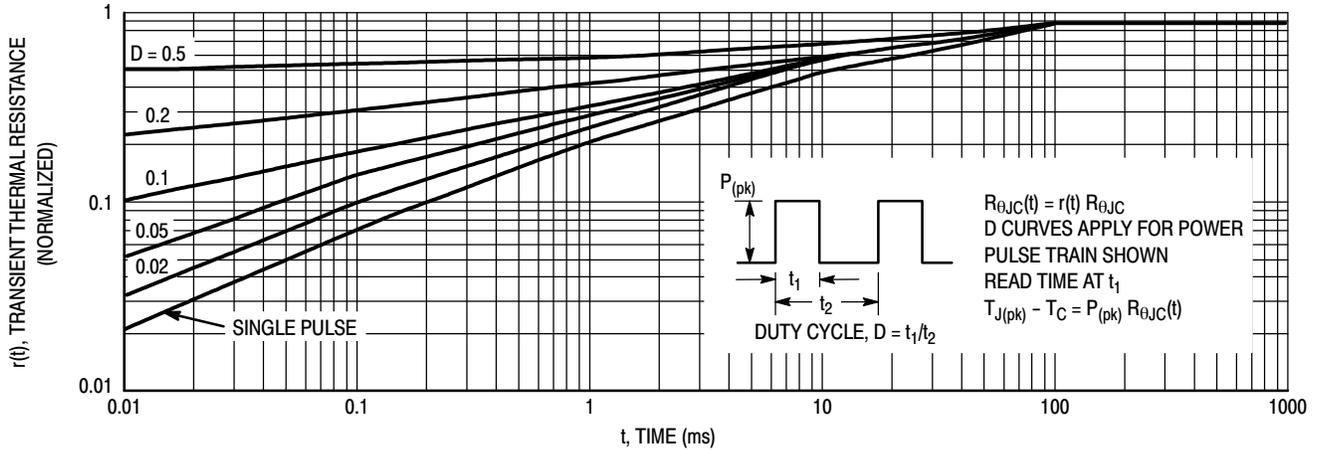
Figure 20. Typical Thermal Response ( $Z_{\theta JC}(t)$ ) for BUL146
