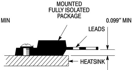
**Figure 22c. Screw Mounting Position for Isolation Test Number 3**
