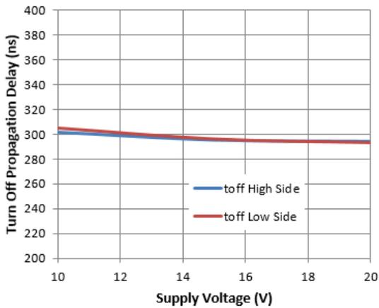
**Figure 7.** Turn-off Propagation Delay vs. Supply Voltage
