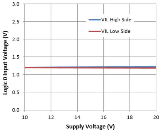
**Figure 23.** Logic 0 Input Voltage vs. Supply Voltage
