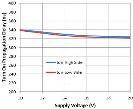
**Figure 5.** Turn-on Propagation Delay vs. Supply Voltage
