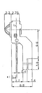
Example of mounting drawing from solder side(Reference)
