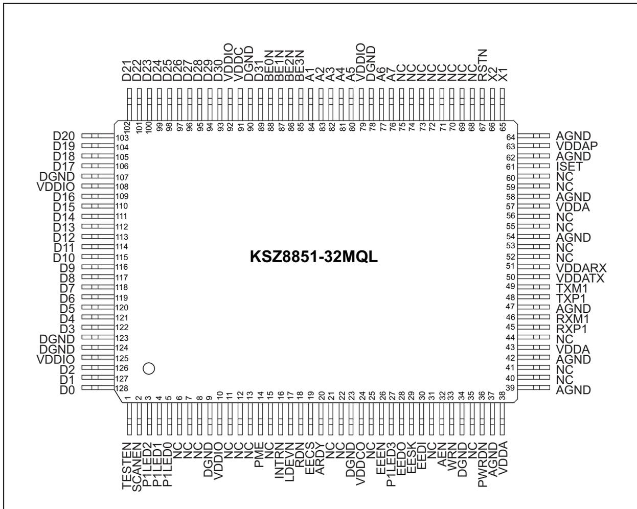
**TABLE 2-2: SIGNALS FOR 32-BIT 128-PIN PQFP**
