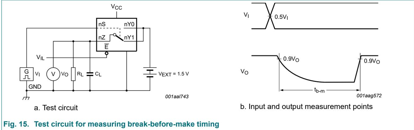
Fig. 15. Test circuit for measuring break-before-make timing
