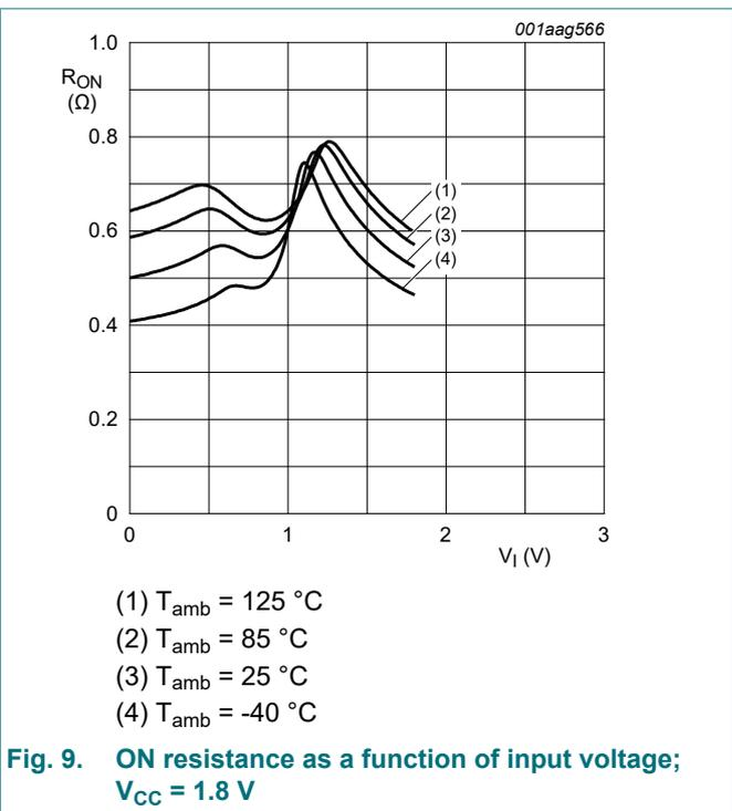
Fig. 9. ON resistance as a function of input voltage; V<sub>CC</sub> = 1.8 V
