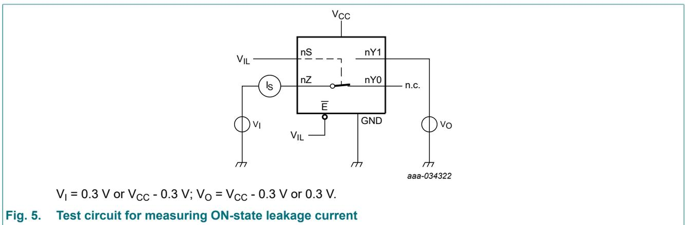
Fig. 5. Test circuit for measuring ON-state leakage current
