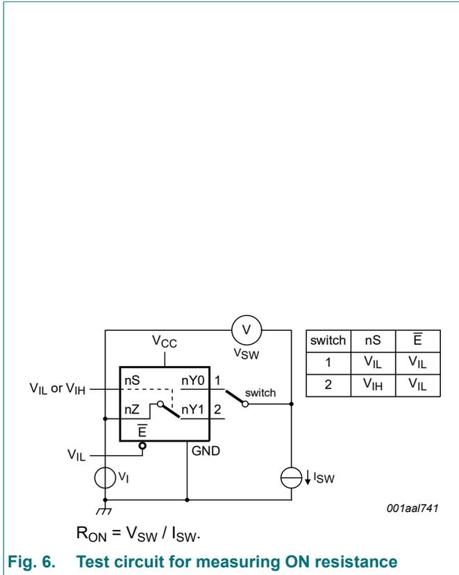
Fig. 6. Test circuit for measuring ON resistance
