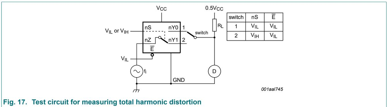
**Fig. 17. Test circuit for measuring total harmonic distortion**
