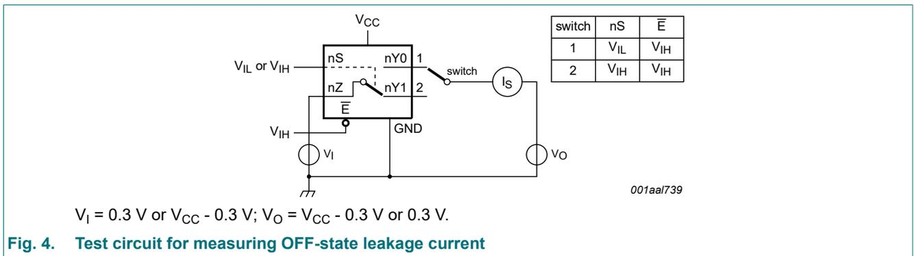
Fig. 4. Test circuit for measuring OFF-state leakage current
