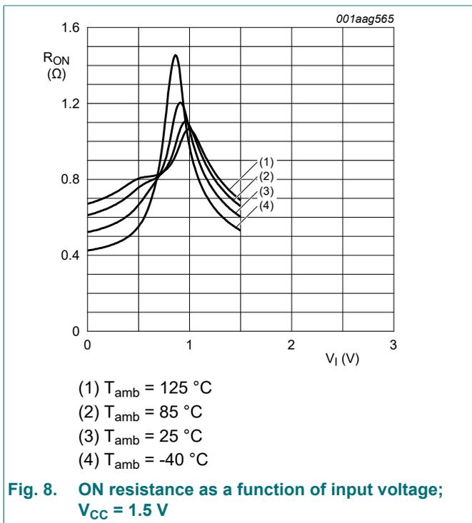
Fig. 8. ON resistance as a function of input voltage; V<sub>CC</sub> = 1.5 V
