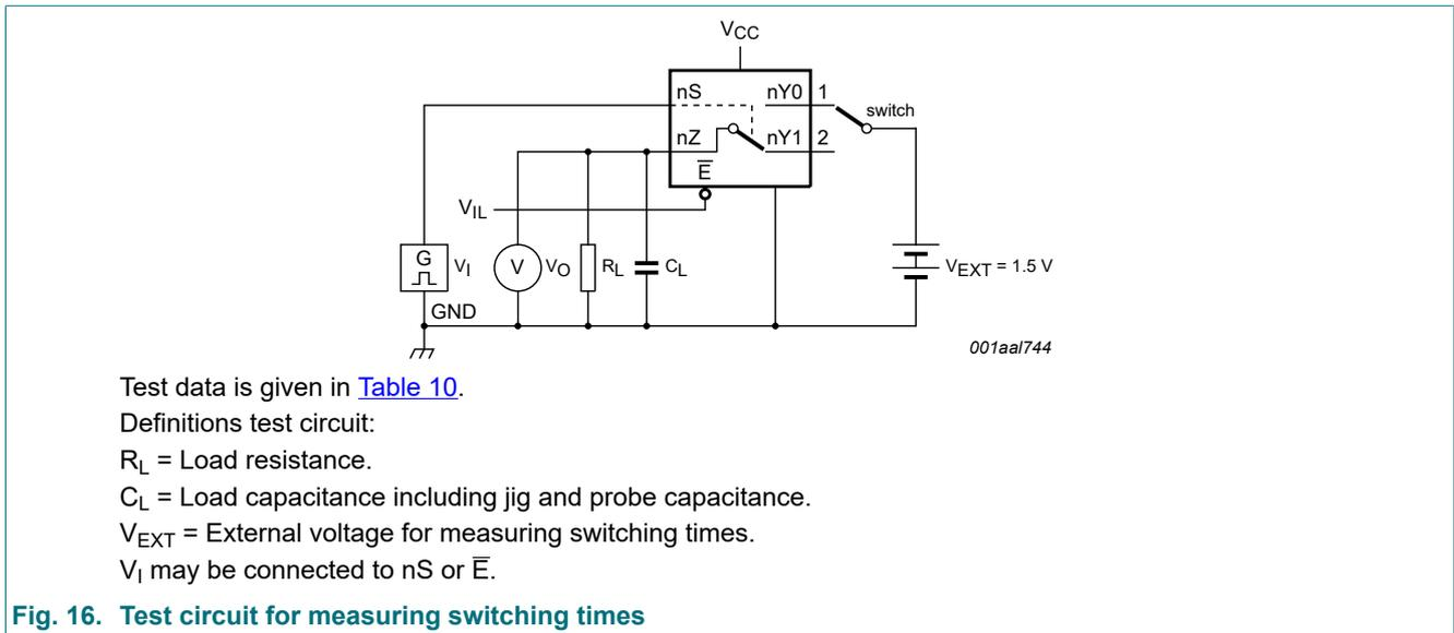
Fig. 16. Test circuit for measuring switching times
