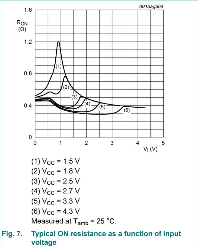
Fig. 7. Typical ON resistance as a function of input voltage
