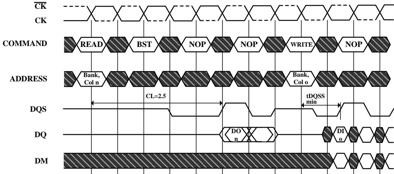
DO<sub>n</sub> (or o) = Data Out from column n (or column o)
