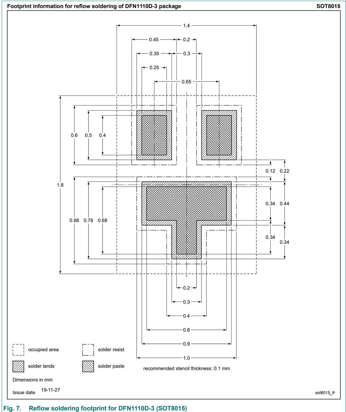
Fig. 7. Reflow soldering footprint for DFN1110D-3 (SOT8015)
