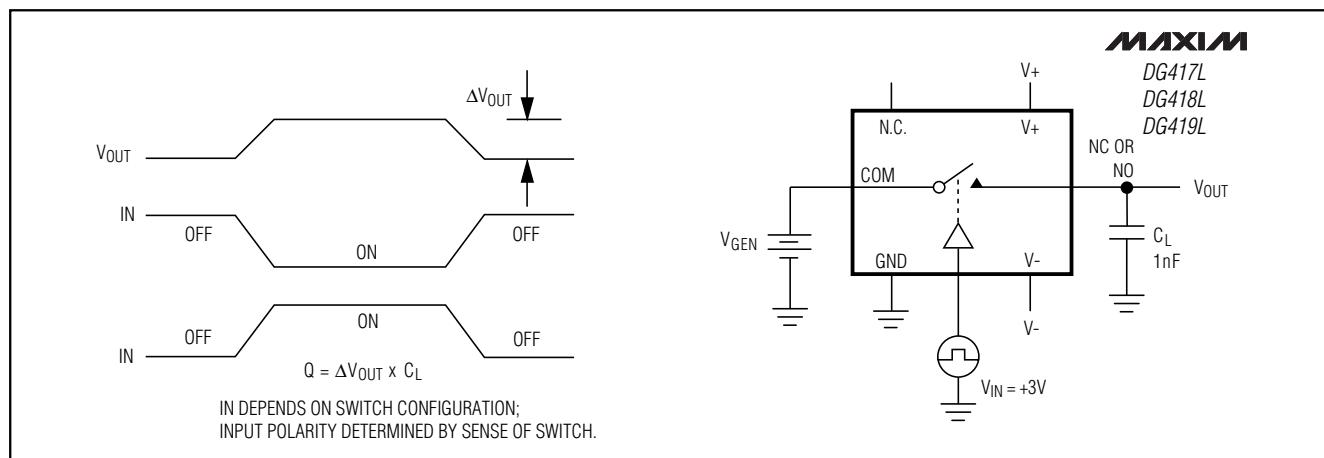
Figure 4. Charge Injection
