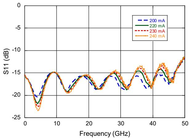
Output Return Loss vs.  $I_{DD}$
