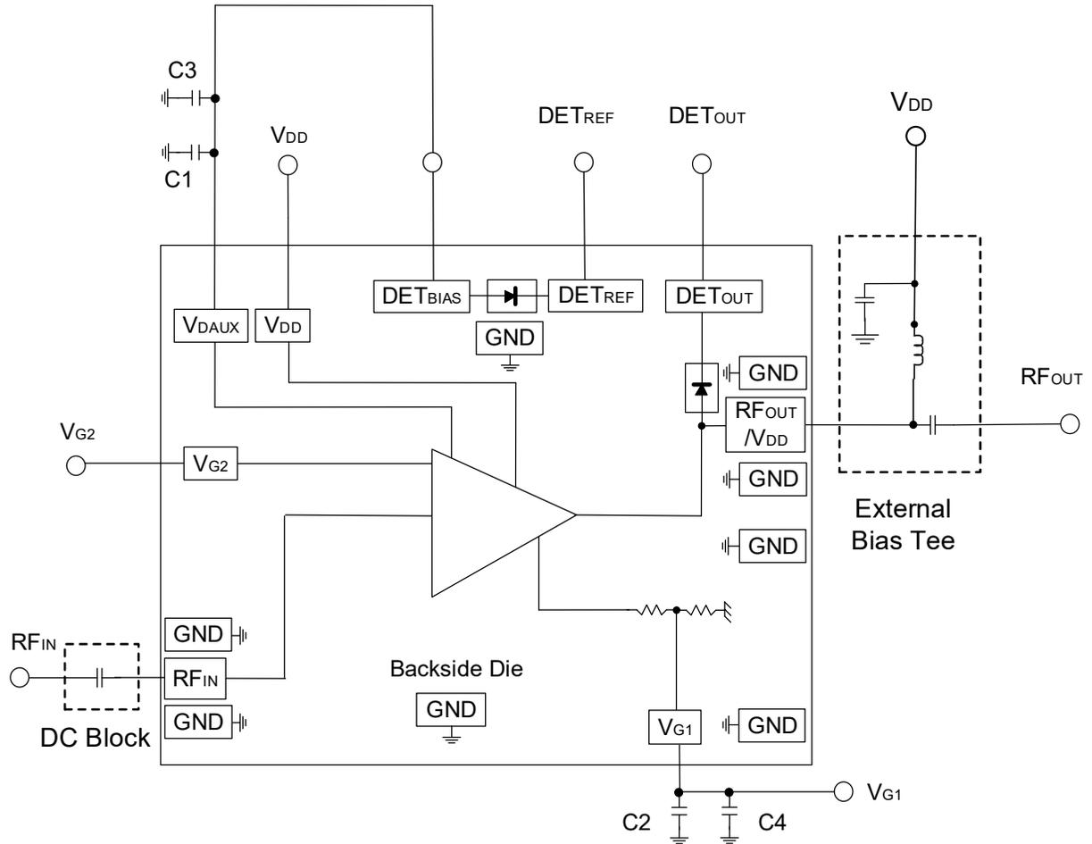
All bond pads labelled GND have vias to the backside metal. Bond wires on these pads are optional.
