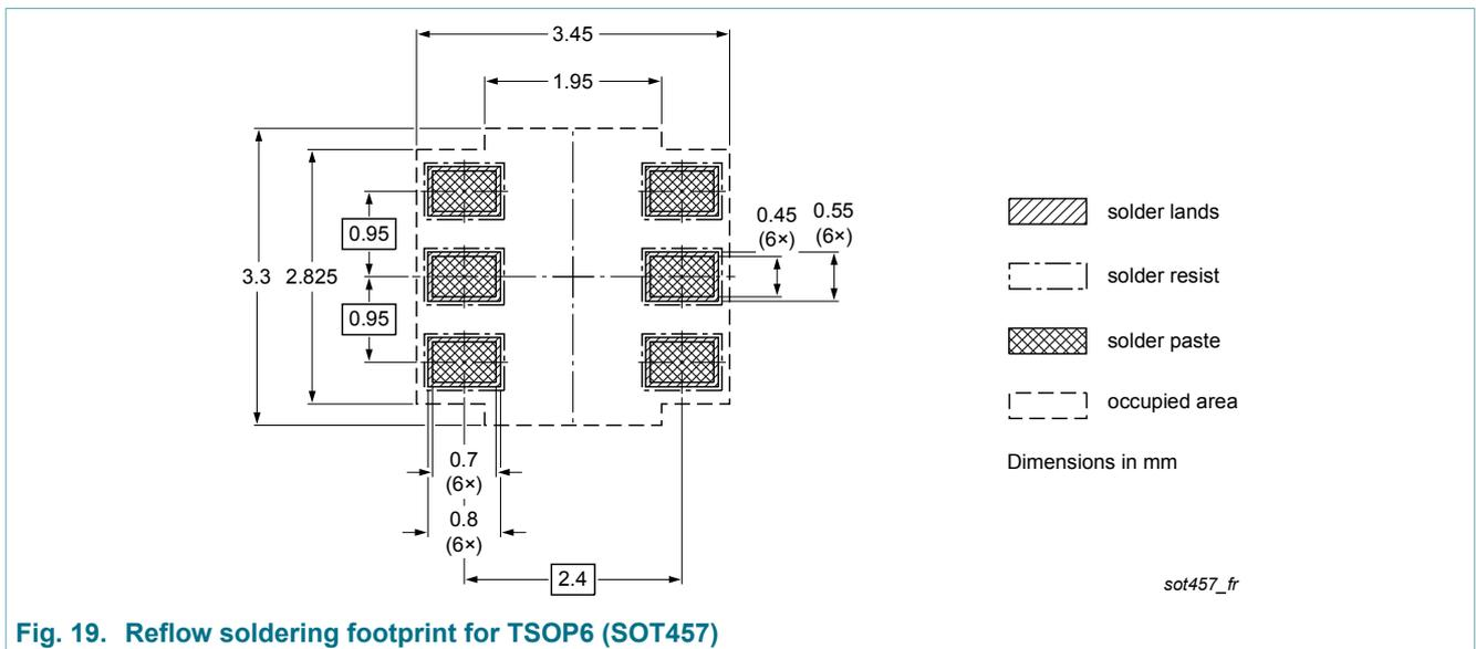
Fig. 19. Reflow soldering footprint for TSOP6 (SOT457)
