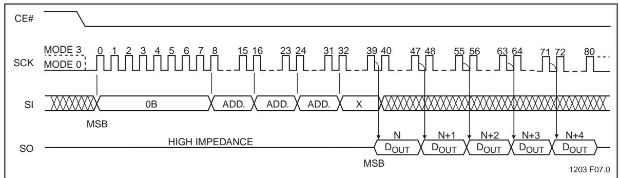
**Figure 8:** High-Speed-Read Sequence
