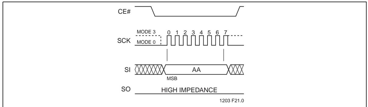
**Figure 22:** Enable-Hold Sequence
