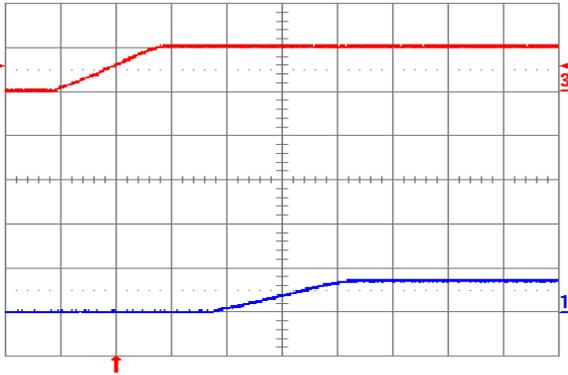
Fig. 0.7525V.5: Turn-on transient for  $V_{out} = 0.7525V$  with application of  $V_{in}$  at full rated load current (resistive) and  $47\mu F$  external capacitance at  $V_{in} = 5V$ . Top trace:  $V_{in}$  (5V/div.); Bottom trace: output voltage (1V/div.); Time scale: 2ms/div.
