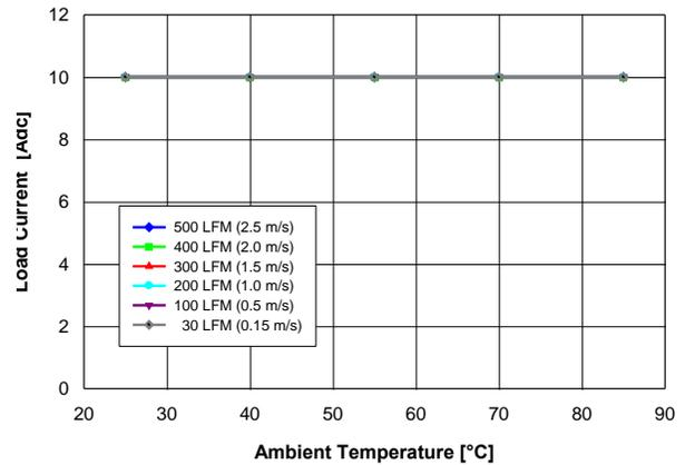
Fig. 1.5V.2: Available load current vs. ambient temperature and airflow rates for  $V_{out} = 1.5V$  converter mounted horizontally with air flowing from pin 10 to pin 1, and maximum MOSFET temperature  $\leq 120^\circ C$ .
