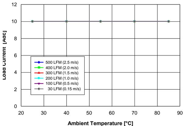
Fig. 1.2V.1: Available load current vs. ambient temperature and airflow rates for  $V_{out} = 1.2V$  converter mounted vertically with air flowing from pin 10 to pin 1, and maximum MOSFET temperature  $\leq 120^\circ C$ .
