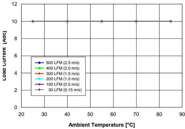
Fig. 2.5V.1: Available load current vs. ambient temperature and airflow rates for  $V_{out} = 2.5V$  converter mounted vertically with air flowing from pin 10 to pin 1, and maximum MOSFET temperature  $\leq 120^\circ C$ .
