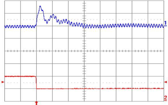
Fig. 3.3V.8: Output voltage response for  $V_{out} = 3.3V$  to negative load current step change from 5A to 2.5A with slew rate of  $-5A/\mu s$  at  $V_{in} = 5V$ . Top trace: output voltage (100mV/div.); Bottom trace: load current (5A/div.).  $C_o = 100\mu F$  ceramic +  $1\mu F$  ceramic. Time scale:  $20\mu s/div$ .
