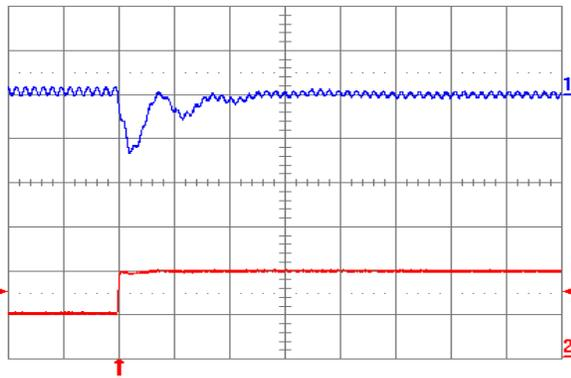
Fig. 2.0V.7: Output voltage response for  $V_{out} = 2.0V$  to positive load current step change from 2.5A to 5A with slew rate of  $5A/\mu s$  at  $V_{in} = 5V$ . Top trace: output voltage (100mV/div.); Bottom trace: load current (5A/div.).  $C_o = 100\mu F$  ceramic +  $1\mu F$  ceramic. Time scale:  $20\mu s$ /div.
