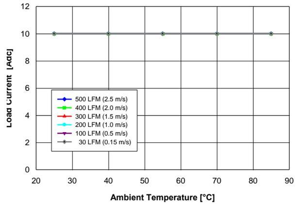
Fig. 0.7525V.2: Available load current vs. ambient temperature and airflow rates for  $V_{out} = 0.7525V$  converter mounted horizontally with air flowing from pin 10 to pin 1, and maximum MOSFET temperature  $\leq 120^\circ C$ .
