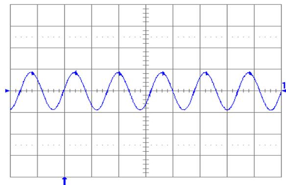
Fig. 3.3V.6: Output voltage ripple (20mV/div.) at full rated load current into a resistive load with external capacitance  $47\mu F$  ceramic +  $1\mu F$  ceramic and  $V_{in} = 5V$  for  $V_{out} = 3.3V$ . Time scale: 2µs/div.
