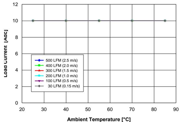
Fig. 1.2V.2: Available load current vs. ambient temperature and airflow rates for  $V_{out} = 1.2V$  converter mounted horizontally with air flowing from pin 10 to pin 1, and maximum MOSFET temperature  $\leq 120^\circ C$ .
