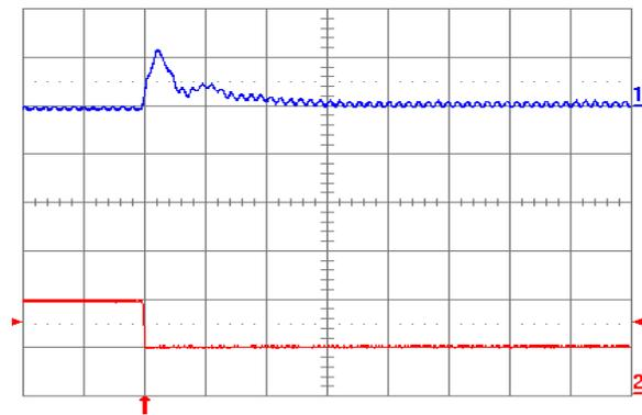
Fig. 1.2V.8: Output voltage response for  $V_{out} = 1.2V$  to negative load current step change from 5A to 2.5A with slew rate of  $-5A/\mu s$  at  $V_{in} = 5V$ . Top trace: output voltage (100mV/div.); Bottom trace: load current (5A/div.).  $C_o = 100\mu F$  ceramic +  $1\mu F$  ceramic. Time scale: 20μs/div.
