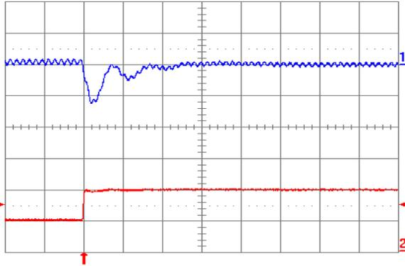
Fig. 1.8V.7: Output voltage response for  $V_{out} = 1.8V$  to positive load current step change from 2.5A to 5A with slew rate of  $5A/\mu s$  at  $V_{in} = 5V$ . Top trace: output voltage (100mV/div.); Bottom trace: load current (5A/div.).  $C_o = 100\mu F$  ceramic +  $1\mu F$  ceramic. Time scale:  $20\mu s/div.$
