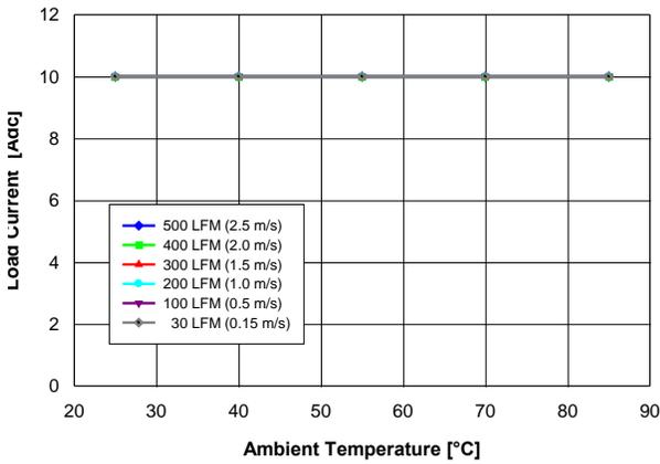
Fig. 0.7525V.1: Available load current vs. ambient temperature and airflow rates for  $V_{out} = 0.7525V$  converter mounted vertically with air flowing from pin 10 to pin 1, and maximum MOSFET temperature  $\leq 120^\circ C$ .
