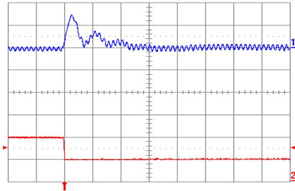
Fig. 2.5V.8: Output voltage response for  $V_{out} = 2.5V$  to negative load current step change from 5A to 2.5A with slew rate of  $-5A/\mu s$  at  $V_{in} = 5V$ . Top trace: output voltage (100mV/div.); Bottom trace: load current (5A/div.).  $C_o = 100\mu F$  ceramic +  $1\mu F$  ceramic. Time scale:  $20\mu s$ /div.
