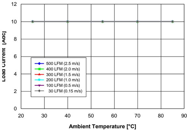
Fig. 1.5V.1: Available load current vs. ambient temperature and airflow rates for  $V_{out} = 1.5V$  converter mounted vertically with air flowing from pin 10 to pin 1, and maximum MOSFET temperature  $\leq 120^\circ C$ .
