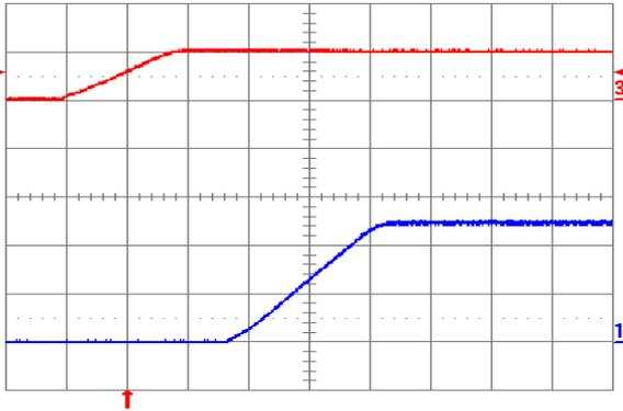
Fig. 2.5V.5: Turn-on transient for  $V_{out} = 2.5V$  with application of  $V_{in}$  at full rated load current (resistive) and  $47\mu F$  external capacitance at  $V_{in} = 5V$ . Top trace:  $V_{in}$  (5V/div.); Bottom trace: output voltage (1V/div.); Time scale: 2ms/div.
