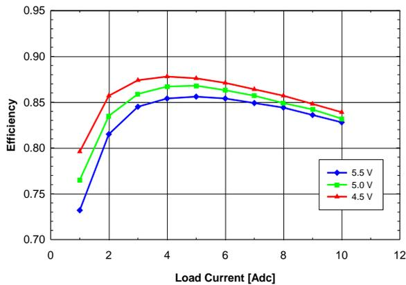
Fig. 0.7525V.3: Efficiency vs. load current and input voltage for  $V_{out} = 0.7525V$  converter mounted vertically with air flowing from pin 10 to pin 1 at a rate of 200 LFM (1m/s) and  $T_a = 25^\circ C$ .
