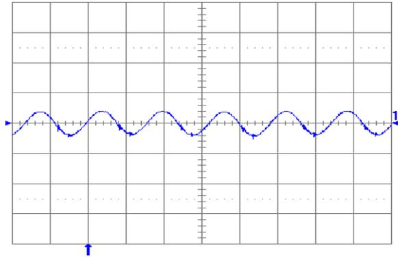
Fig. 0.7525V.6: Output voltage ripple (20mV/div.) at full rated load current into a resistive load with external capacitance  $47\mu F$  ceramic +  $1\mu F$  ceramic and  $V_{in} = 5V$  for  $V_{out} = 0.7525V$ . Time scale: 2 $\mu s$ /div.
