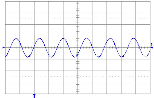
Fig. 1.8V.6: Output voltage ripple (20mV/div.) at full rated load current into a resistive load with external capacitance  $47\mu F$  ceramic +  $1\mu F$  ceramic and  $V_{in} = 5V$  for  $V_{out} = 1.8V$ . Time scale: 2µs/div.
