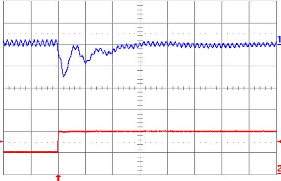
Fig. 3.3V.7: Output voltage response for  $V_{out} = 3.3V$  to positive load current step change from 2.5A to 5A with slew rate of  $5A/\mu s$  at  $V_{in} = 5V$ . Top trace: output voltage (100mV/div.); Bottom trace: load current (5A/div.).  $C_o = 100\mu F$  ceramic +  $1\mu F$  ceramic. Time scale:  $20\mu s/div$ .
