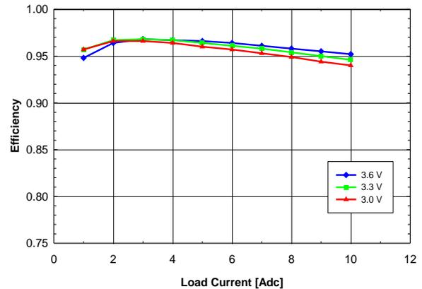
Fig. 2.5V.4: Efficiency vs. load current and input voltage for  $V_{out} = 2.5V$  converter mounted horizontally with air flowing from pin 10 to pin 1 at a rate of 200 LFM (1m/s) and  $T_a = 25^\circ C$ .
