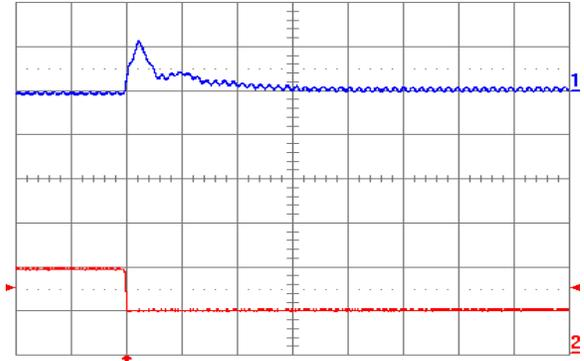
Fig. 1.0V.8: Output voltage response for  $V_{out} = 1.0V$  to negative load current step change from 5A to 2.5A with slew rate of  $-5A/\mu s$  at  $V_{in} = 5V$ . Top trace: output voltage (100mV/div.); Bottom trace: load current (5A/div.).  $C_o = 100\mu F$  ceramic +  $1\mu F$  ceramic. Time scale:  $20\mu s/div.$
