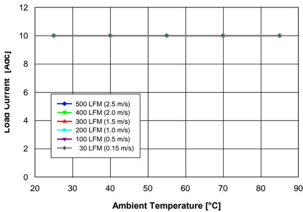
Fig. 3.3V.1: Available load current vs. ambient temperature and airflow rates for  $V_{out} = 3.3V$  converter mounted vertically with  $V_{in} = 5V$ , air flowing from pin 10 to pin 1, and maximum MOSFET temperature  $\leq 120^{\circ}C$ .
