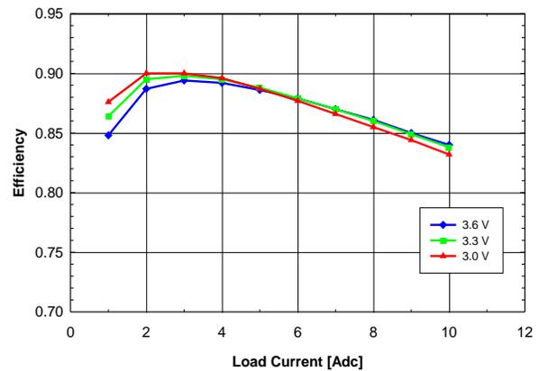
Fig. 0.7525V.4: Efficiency vs. load current and input voltage for  $V_{out} = 0.7525V$  converter mounted vertically with air flowing from pin 10 to pin 1 at a rate of 200 LFM (1m/s) and  $T_a = 25^\circ C$ .
