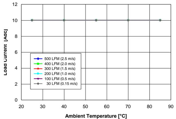
Fig. 2.0V.2: Available load current vs. ambient temperature and airflow rates for  $V_{out} = 2.0V$  converter mounted horizontally with air flowing from pin 10 to pin 1, and maximum MOSFET temperature  $\leq 120^\circ C$ .
