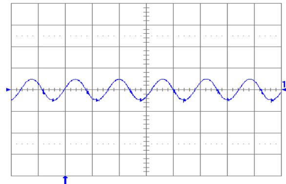
Fig. 1.0V.6: Output voltage ripple (20mV/div.) at full rated load current into a resistive load with external capacitance  $47\mu F$  ceramic +  $1\mu F$  ceramic and  $V_{in} = 5V$  for  $V_{out} = 1.0V$ . Time scale: 2µs/div.
