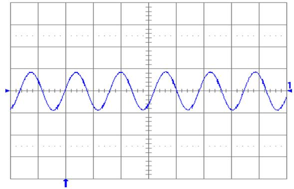
Fig. 2.0V.6: Output voltage ripple (20mV/div.) at full rated load current into a resistive load with external capacitance  $47\mu F$  ceramic +  $1\mu F$  ceramic and  $V_{in} = 5V$  for  $V_{out} = 2.0V$ . Time scale:  $2\mu s$ /div.
