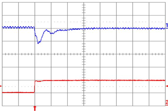
Fig. 1.2V.7: Output voltage response for  $V_{out} = 1.2V$  to positive load current step change from 2.5A to 5A with slew rate of  $5A/\mu s$  at  $V_{in} = 5V$ . Top trace: output voltage (100mV/div.); Bottom trace: load current (5A/div.).  $C_o = 100\mu F$  ceramic +  $1\mu F$  ceramic. Time scale: 20μs/div.
