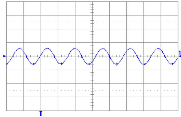
Fig. 1.2V.6: Output voltage ripple (20mV/div.) at full rated load current into a resistive load with external capacitance  $47\mu F$  ceramic +  $1\mu F$  ceramic and  $V_{in} = 5V$  for  $V_{out} = 1.2V$ . Time scale: 2μs/div.
