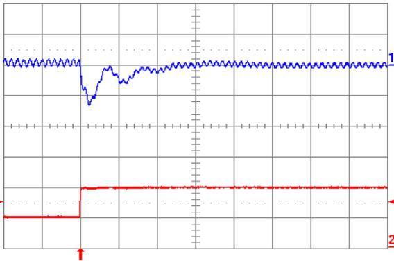
Fig. 2.5V.7: Output voltage response for  $V_{out} = 2.5V$  to positive load current step change from 2.5A to 5A with slew rate of  $5A/\mu s$  at  $V_{in} = 5V$ . Top trace: output voltage (100mV/div.); Bottom trace: load current (5A/div.).  $C_o = 100\mu F$  ceramic +  $1\mu F$  ceramic. Time scale:  $20\mu s$ /div.
