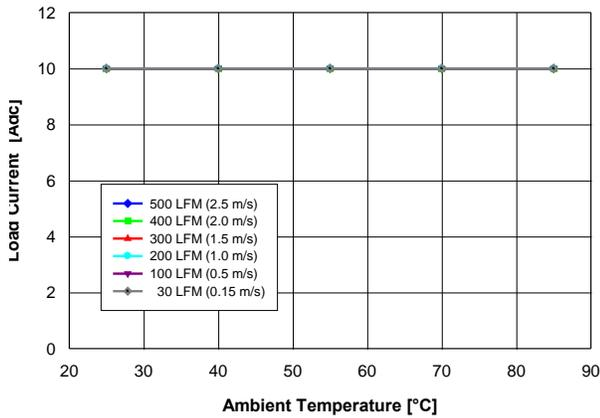
Fig. 1.0V.1: Available load current vs. ambient temperature and airflow rates for  $V_{out} = 1.0V$  converter mounted vertically with air flowing from pin 10 to pin 1, and maximum MOSFET temperature  $\leq 120^{\circ}C$ .
