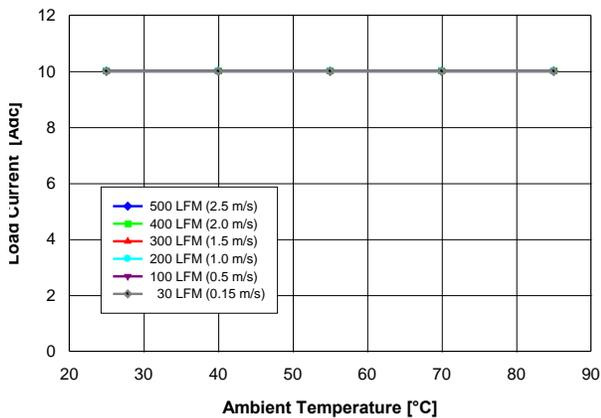
Fig. 2.0V.1: Available load current vs. ambient temperature and airflow rates for  $V_{out} = 2.0V$  converter mounted vertically with air flowing from pin 10 to pin 1, and maximum MOSFET temperature  $\leq 120^\circ C$ .
