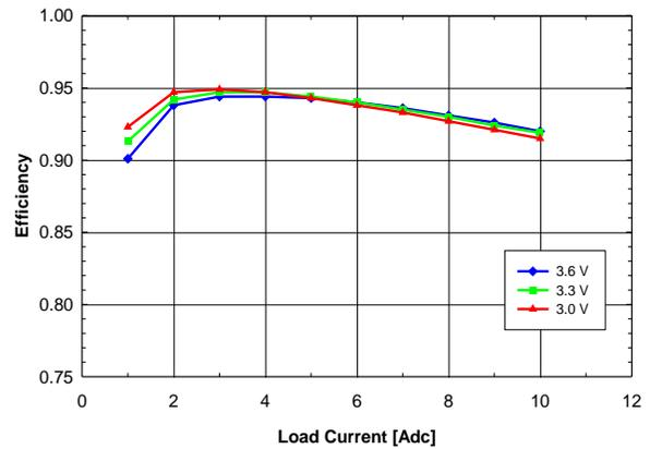
Fig. 1.8V.4: Efficiency vs. load current and input voltage for  $V_{out} = 1.8V$  converter mounted horizontally with air flowing from pin 10 to pin 1 at a rate of 200 LFM (1m/s) and  $T_a = 25^{\circ}C$ .
