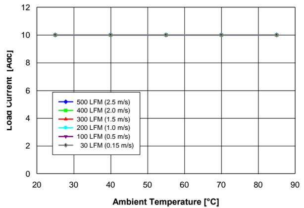
Fig. 3.3V.2: Available load current vs. ambient temperature and airflow rates for  $V_{out} = 3.3V$  converter mounted horizontally with  $V_{in} = 5V$ , air flowing from pin 10 to pin 1, and maximum MOSFET temperature  $\leq 120^{\circ}C$ .
