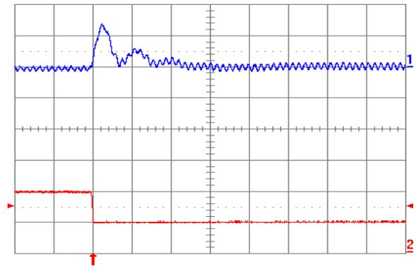
Fig. 2.0V.8: Output voltage response for  $V_{out} = 2.0V$  to negative load current step change from 5A to 2.5A with slew rate of  $-5A/\mu s$  at  $V_{in} = 5V$ . Top trace: output voltage (100mV/div.); Bottom trace: load current (5A/div.).  $C_o = 100\mu F$  ceramic +  $1\mu F$  ceramic. Time scale:  $20\mu s$ /div.
