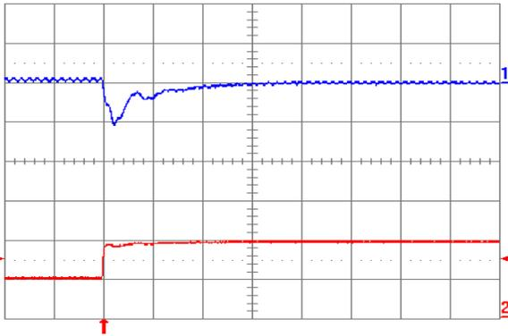
Fig. 0.7525V.7: Output voltage response for  $V_{out} = 0.7525V$  to positive load current step change from 2.5A to 5A with slew rate of  $5A/\mu s$  at  $V_{in} = 5V$ . Top trace: output voltage (100mV/div.); Bottom trace: load current (5A/div.).  $C_o = 100\mu F$  ceramic +  $1\mu F$  ceramic. Time scale: 20 $\mu s$ /div.
