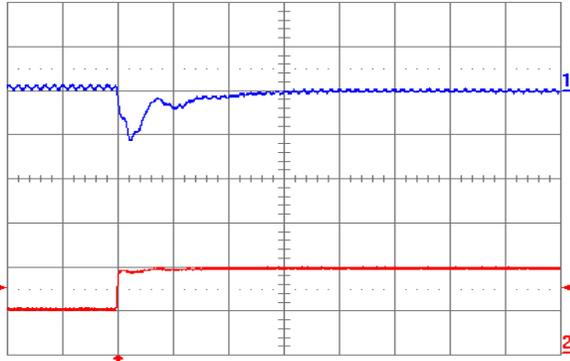
Fig. 1.0V.7: Output voltage response for  $V_{out} = 1.0V$  to positive load current step change from 2.5A to 5A with slew rate of  $5A/\mu s$  at  $V_{in} = 5V$ . Top trace: output voltage (100mV/div.); Bottom trace: load current (5A/div.).  $C_o = 100\mu F$  ceramic +  $1\mu F$  ceramic. Time scale:  $20\mu s/div.$
