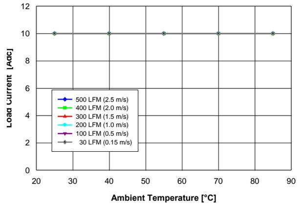
Fig. 1.0V.2: Available load current vs. ambient temperature and airflow rates for  $V_{out} = 1.0V$  converter mounted horizontally with air flowing from pin 10 to pin 1, and maximum MOSFET temperature  $\leq 120^{\circ}C$ .
