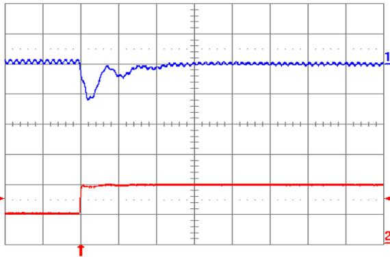
Fig. 1.5V.7: Output voltage response for  $V_{out} = 1.5V$  to positive load current step change from 2.5A to 5A with slew rate of  $5A/\mu s$  at  $V_{in} = 5V$ . Top trace: output voltage (100mV/div.); Bottom trace: load current (5A/div.).  $C_o = 100\mu F$  ceramic +  $1\mu F$  ceramic. Time scale:  $20\mu s$ /div.
