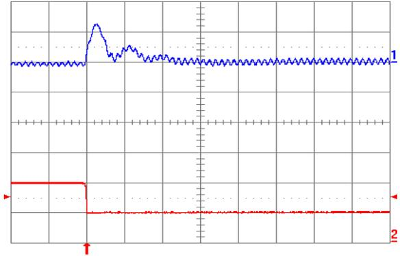
Fig. 1.8V.8: Output voltage response for  $V_{out} = 1.8V$  to negative load current step change from 5A to 2.5A with slew rate of  $-5A/\mu s$  at  $V_{in} = 5V$ . Top trace: output voltage (100mV/div.); Bottom trace: load current (5A/div.).  $C_o = 100\mu F$  ceramic +  $1\mu F$  ceramic. Time scale:  $20\mu s/div.$
