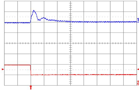
Fig. 0.7525V.8: Output voltage response for  $V_{out} = 0.7525V$  to negative load current step change from 5A to 2.5A with slew rate of  $-5A/\mu s$  at  $V_{in} = 5V$ . Top trace: output voltage (100mV/div.); Bottom trace: load current (5A/div.).  $C_o = 100\mu F$  ceramic +  $1\mu F$  ceramic. Time scale: 20 $\mu s$ /div.
