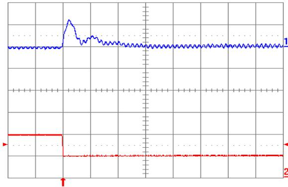
Fig. 1.5V.8: Output voltage response for  $V_{out} = 1.5V$  to negative load current step change from 5A to 2.5A with slew rate of  $-5A/\mu s$  at  $V_{in} = 5V$ . Top trace: output voltage (100mV/div.); Bottom trace: load current (5A/div.).  $C_o = 100\mu F$  ceramic +  $1\mu F$  ceramic. Time scale:  $20\mu s$ /div.
