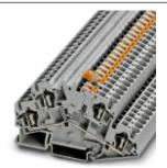
Knife disconnect terminal block, Cross section: 0.08 mm² - 6 mm², AWG: 28 - 10, Connection type: Spring-cage connection, Width: 6.2 mm, Color: blue, Mounting type: NS 35/7,5, NS 35/15
