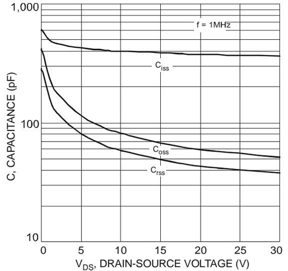
Fig. 6 Typical Capacitance
