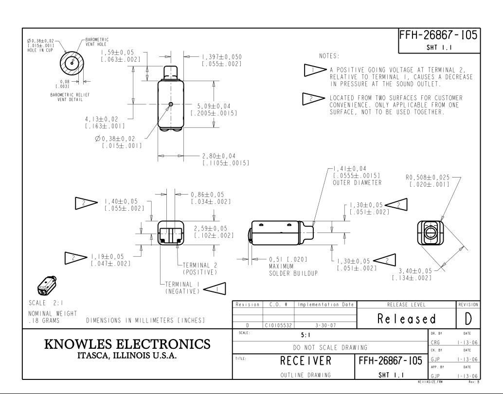
THE FFH-26867-105 IS A FERROFLUID AND TYPE III DAMPED AND EXTERNALLY VENTED FH-26555 RECEIVER WITH A PEAK OF 5dB RELATIVE TO THE SENSITIVITY AT IKHZ UNDER CONSTANT VOLTAGE DRIVE CONDITIONS.
