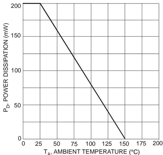
Fig. 1, Power Dissipation vs. Ambient Temperature (Total Device)
