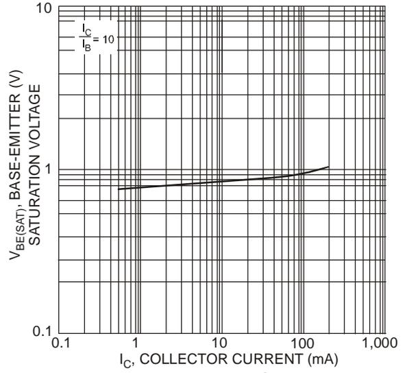
Fig. 5, Typical Base-Emitter Saturation Voltage vs. Collector Current
