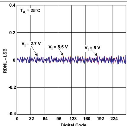
Figure 8. Rheostat Mode RDNL vs Digital Code (25°C)
