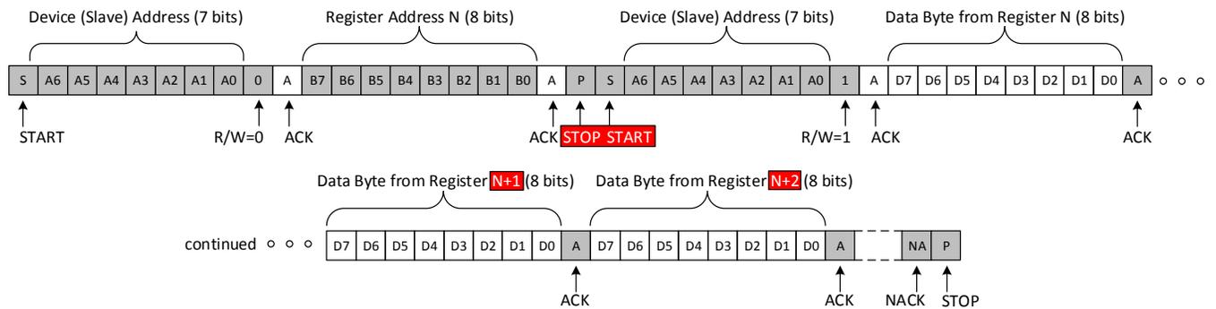
Read from multiple registers in a device (Repeated Start)
