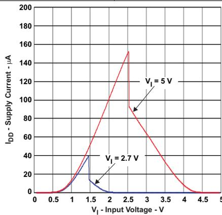
Figure 17. Supply Current vs Digital Input Voltage
