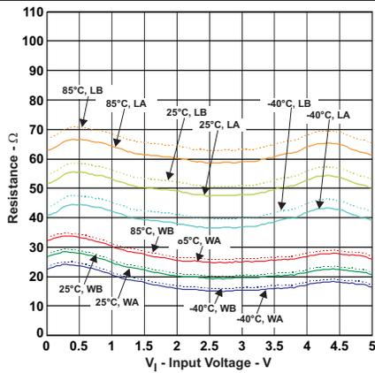
Figure 15. Wiper to Low Terminal Resistance ( $V_{DD} = 5\text{ V}$ )
