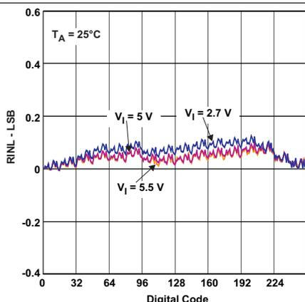
Figure 7. Rheostat Mode RINL vs Digital Code (25°C)
