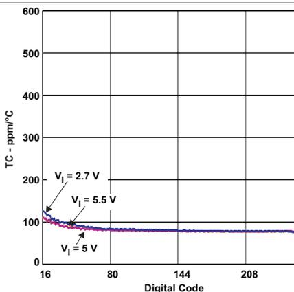
Figure 9. Rheostat Mode  $TC_R$  vs Digital Code
