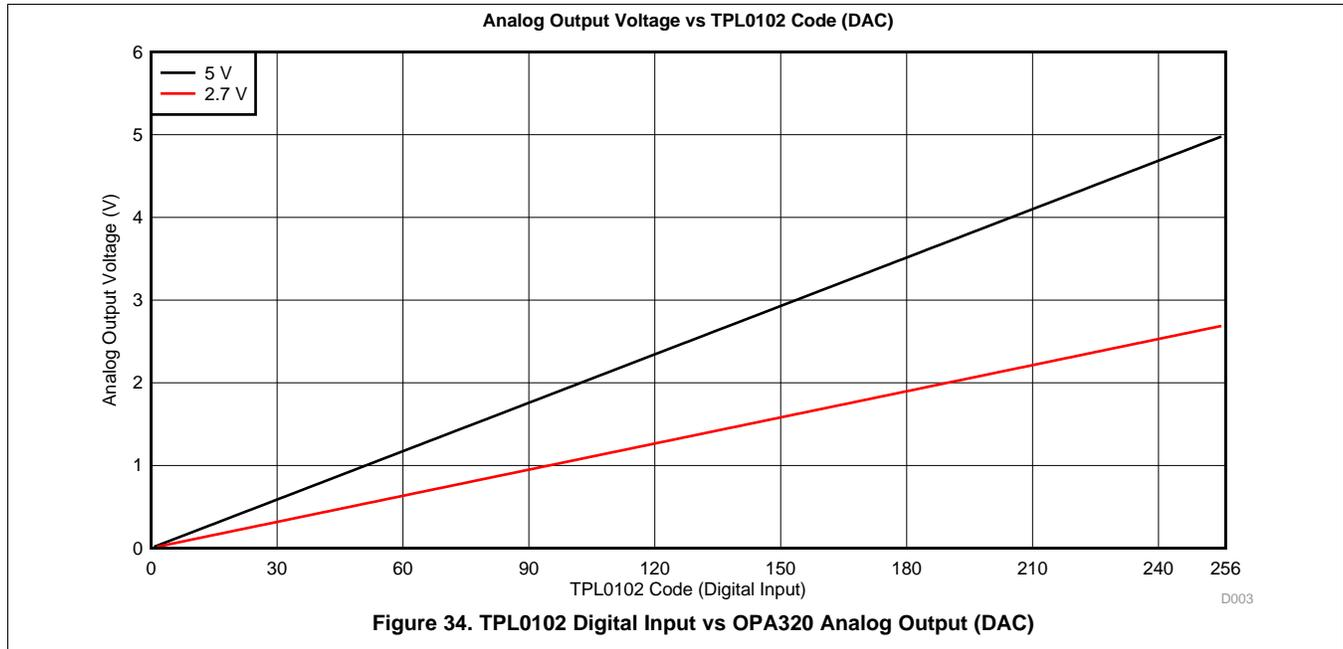
**Figure 34. TPL0102 Digital Input vs OPA320 Analog Output (DAC)**
