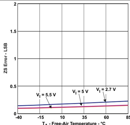
Figure 12. Voltage Divider Mode ZS Error vs Temperature
