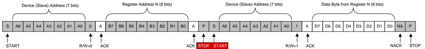
Read from one register in a device (Repeated Start)
