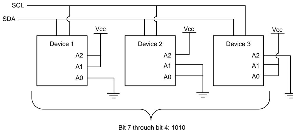
**Figure 30. Examples of Device Address Configuration on I<sup>2</sup>C Bus**
