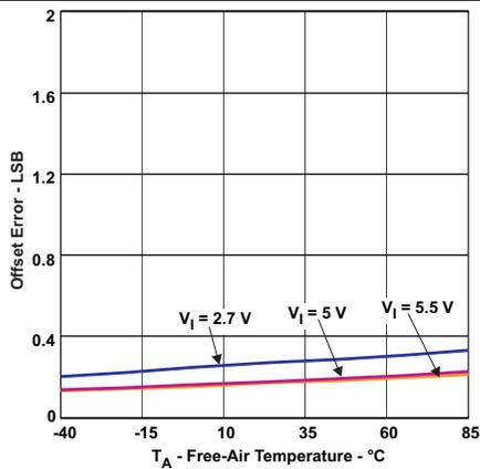
Figure 13. Rheostat Mode Offset Error vs Temperature
