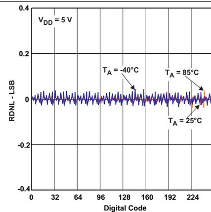
Figure 6. Rheostat Mode RDNL vs Digital Code ( $V_{DD} = 5$  V)
