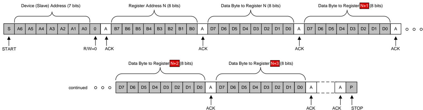
Figure 26. Write Operation to One or Multiple Registers
