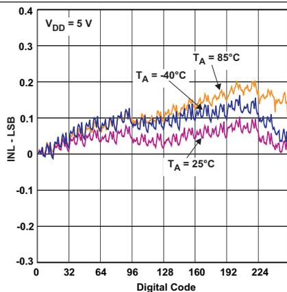
Figure 5. Rheostat Mode RINL vs Digital Code ( $V_{DD} = 5$  V)
