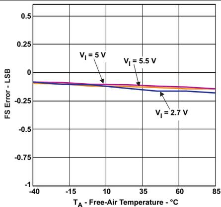
Figure 11. Voltage Divider Mode FS Error vs Temperature
