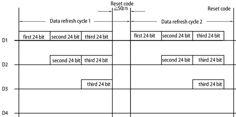
Note: The data of D1 is sent by MCU, and D2,D3,D4 through pixel internal reshaping amplification to transmit.
