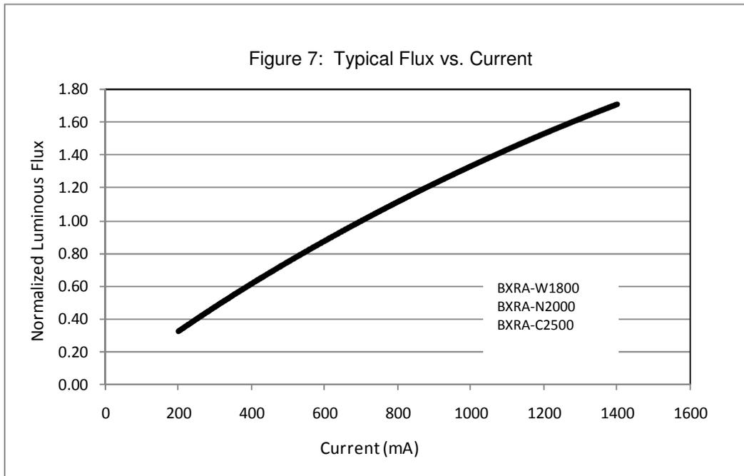
Note for Figure 7: Bridgelux does not recommend driving high power LED Arrays at low currents. Doing so may produce unpredictable results. Pulse width modulation (PWM) is recommended for dimming effects.
