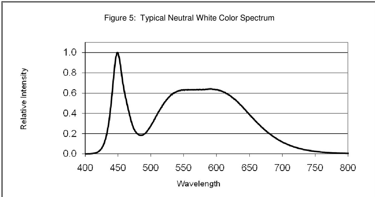
Wavelength Characteristics at Rated Test Current,  $T_j=25^\circ\text{C}$  (Continued)
