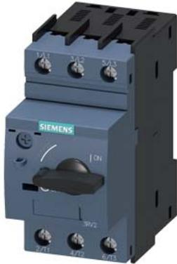
Circuit breaker size S00 for motor protection, CLASS 10 A-release 1.1...1.6 A N-release 21 A screw terminal Standard switching capacity
