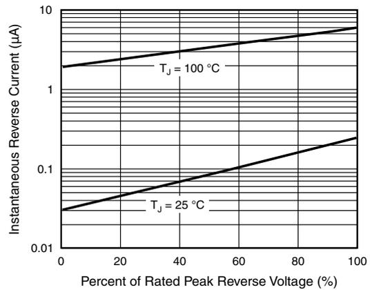
Fig. 5 - Typical Reverse Leakage Characteristics Per Diode
