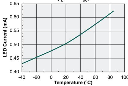
Load Current vs. Load Temperature
