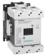
Electrically held lighting contactor, Contactor amp rating 300A, 0 N.C. / 3 N.O. Poles, 208VAC 50/60HZ coil, Non-combination type, (no disconnect device), Enclosure NEMA type (open), No enclosure
