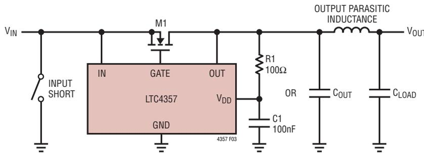
Figure 3. Protecting Against Collapse of V<sub>DD</sub> During Reverse Recovery
