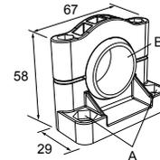
Hole center spacing: A= $\varnothing$  50.8
