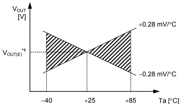
\*1.  $V_{OUT(E)}$  is the value of the output voltage measured at  $T_a = +25^{\circ}\text{C}$ .
