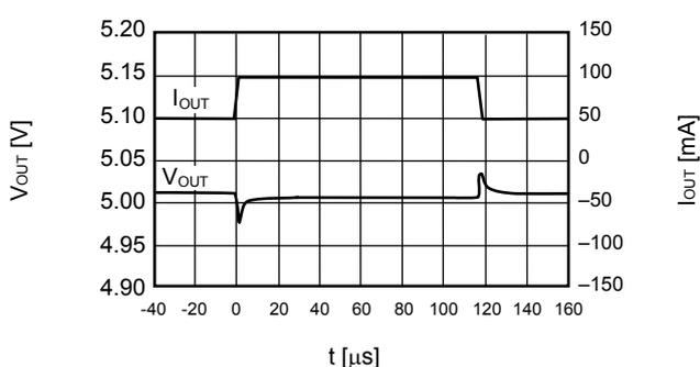
**(3) ON/OFF pin transient response characteristics**
