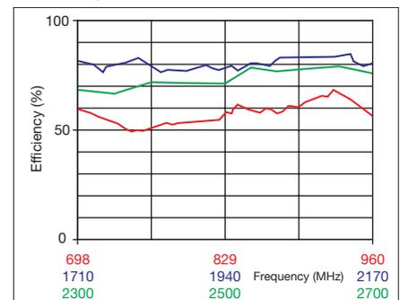
**698-960, 1710-2170 & 2300-2700 MHz LTE/Cell Band Antenna**
