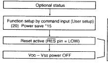
Set the time (t) from reset active to turning off the VDD - Vss power (VDD - Vss = 1.8 V) longer than the time ( $t_H$ ) when the potential of V5 ~ V1 becomes below the threshold voltage (approximately 1 V) of the LCD panel. For th, refer to the <Reference Data> of this event. When this too long, insert a resistor between Vs and Vpp to reduce it.
