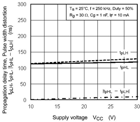
**Fig. 12.2.13**  $t_{pLH}, t_{pHL}, |t_{pHL} - t_{pLH}| - V_{CC}$
