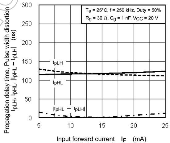
**Fig. 12.2.12  $t_{pLH}, t_{pHL}, |t_{pHL} - t_{pLH}| - I_F$**
