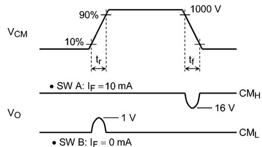
Fig. 12.1.8 Common-Mode Transient Immunity Test Circuit and Waveform
